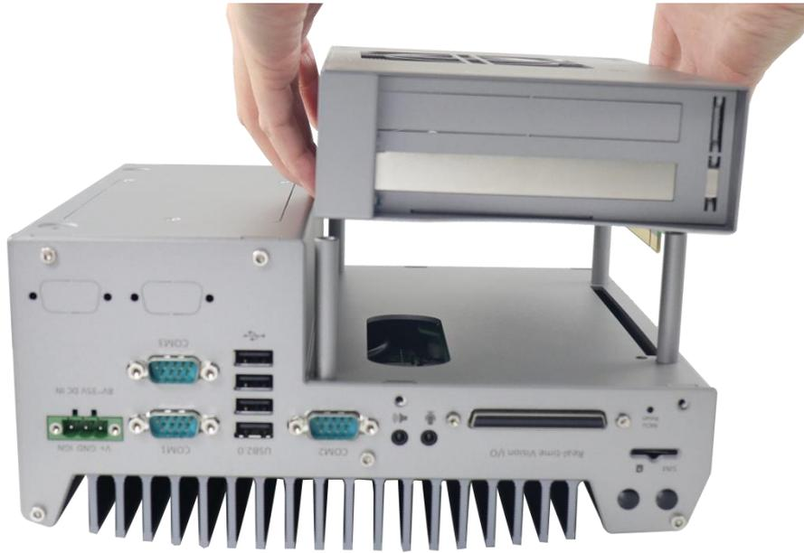
5. Secure the Cassette module by securing the four (4) screws.
