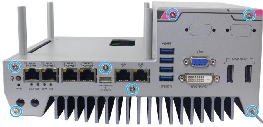
3. Secure the seven (7) screws on the rear panel.
